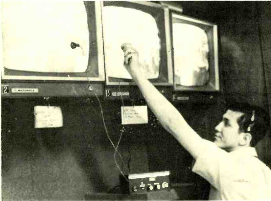
SENSORS PLACED ON MONITOR SCREENS detect changes in light intensity, indicating presence of some person in the area being watched. This system is particularly useful after sales hours. At Macy's, cameras scan stockrooms, corridors and sales areas for prowlers who stay in store after closing and steal by night. Now, any movement in normally quiet area will be detected and a patrol or guard/dog team will be alerted.
